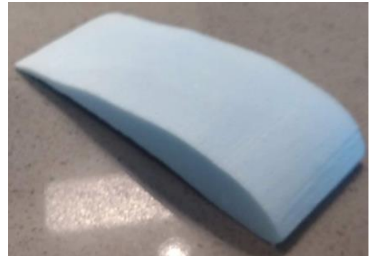
Figure 14: A 3" foam cut section of the S1223 airfoil
